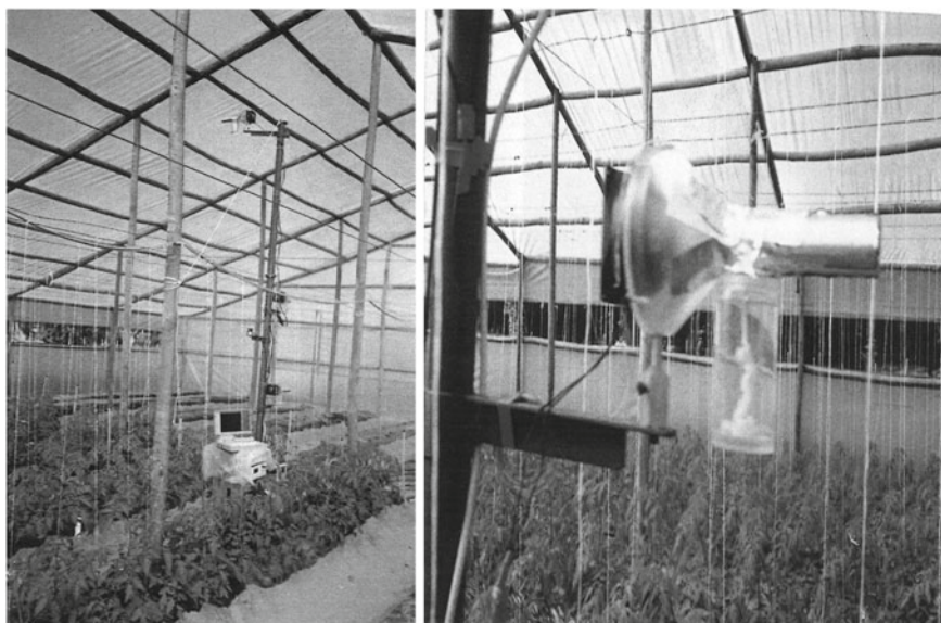
Fig. 6.10 Instrumentation for calculating leaf transpiration in tomato greenhouse. Left: an instrumented mast for data acquisition. Right: An aspiration hygrometer (adapt. Rodrigues 1993)
