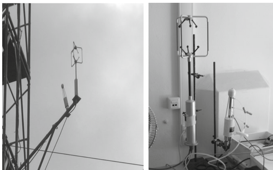
Fig. 3.11 Sonic anemometer and open-path carbon and water vapour analyser (left), with close-up view (right) installed in the field
